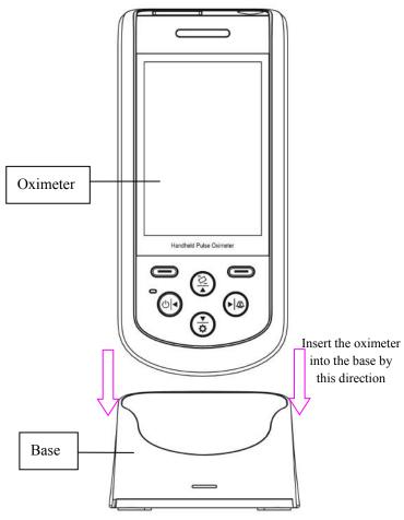
Figure 2.2 Connection between oximeter and base
