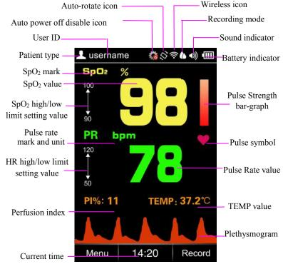
Figure 4.2A Default Display Screen---in vertical **Description:**
