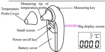
Figure 3.2 the infrared temperature probe
